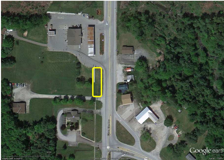
Figure 3. Potential location for stormwater treatment along the west side of Route 7, north of VT Route 104A, between the People's Trust Bank and the Mobil gas station.
